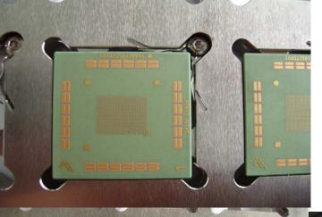
Interchangeable springs pushes all BGA to one uniform corner for precision locating.
